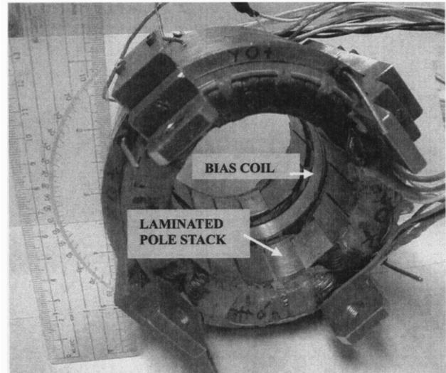
Fig. 5 Homopolar bearing for position stiffness measurements
