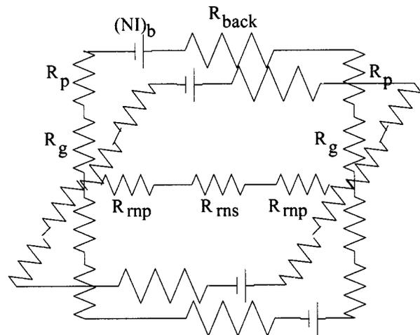
Fig. 4 Homopolar bearing bias path circuit model
