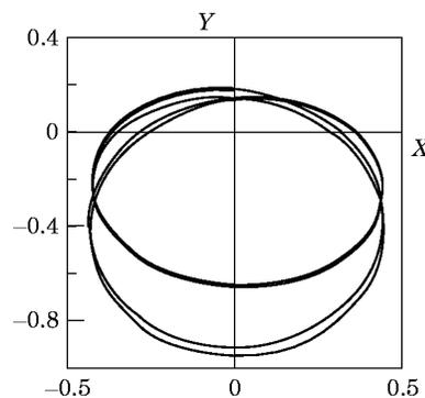
Figure 11. Period-4 orbit;  $P = 1:1$ ,  $D = 0.03$ ,  $G = 0.03$ ,  $\Omega = 1$ ,  $\alpha = 0.16$ .
